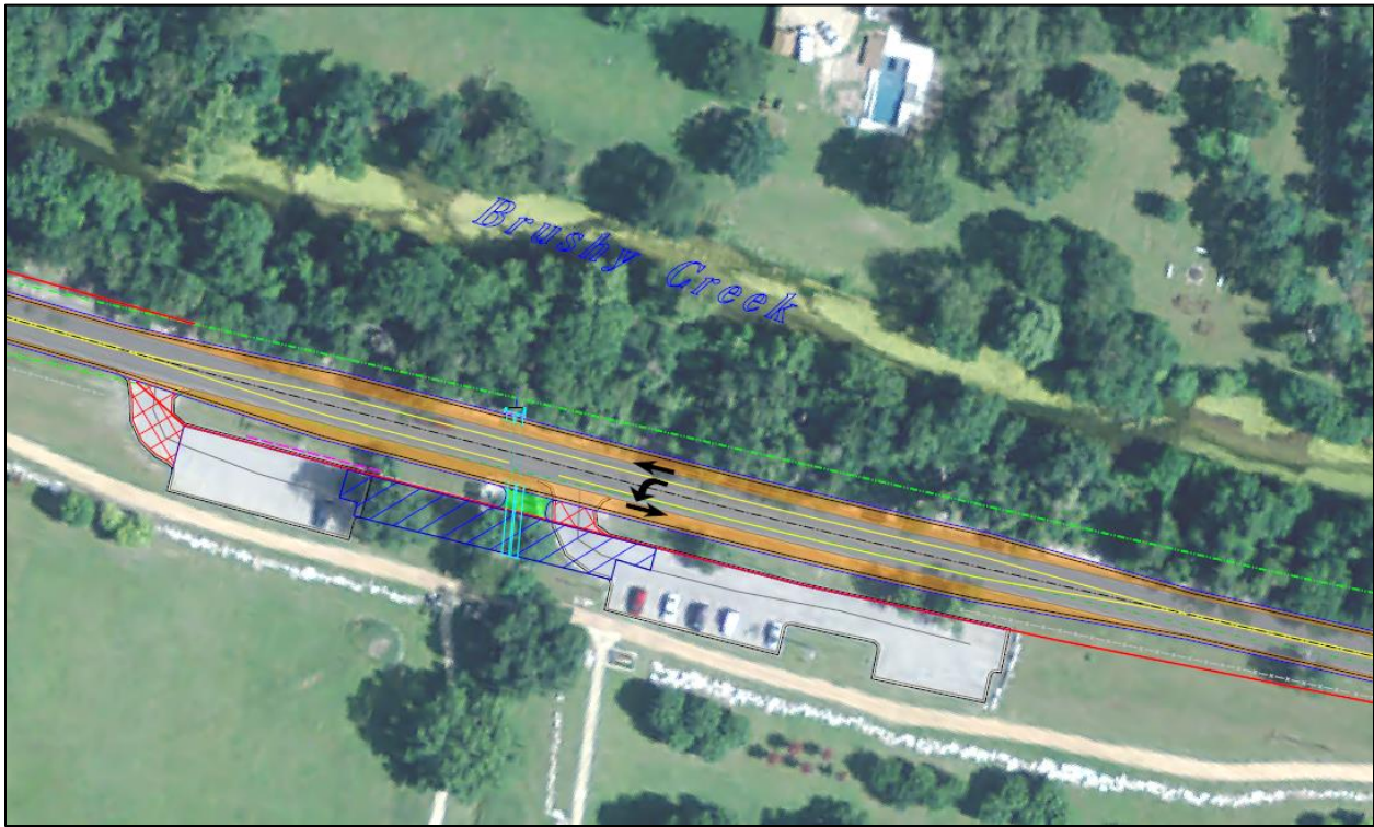
Proposed left-turn lanes into park facilities and widened shoulders along Hairy Man Rd.
